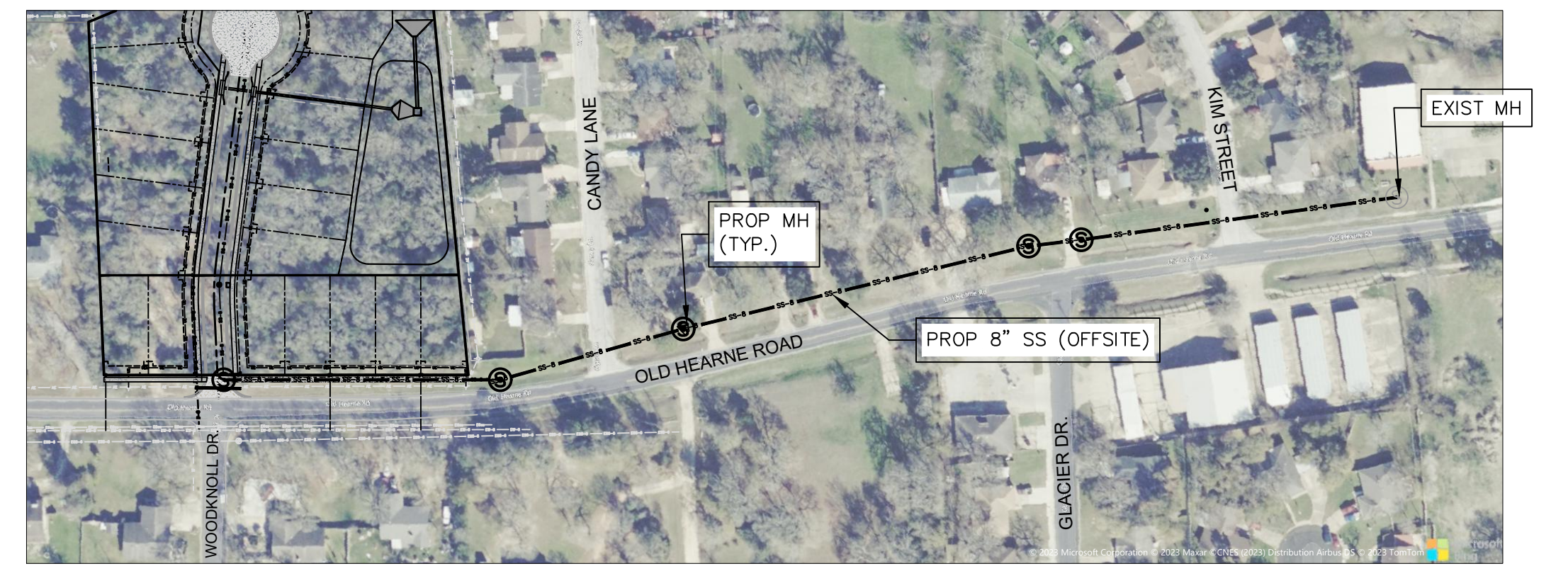
OFF-SITE SANITARY SEWER SCALE: 1" = 150'
